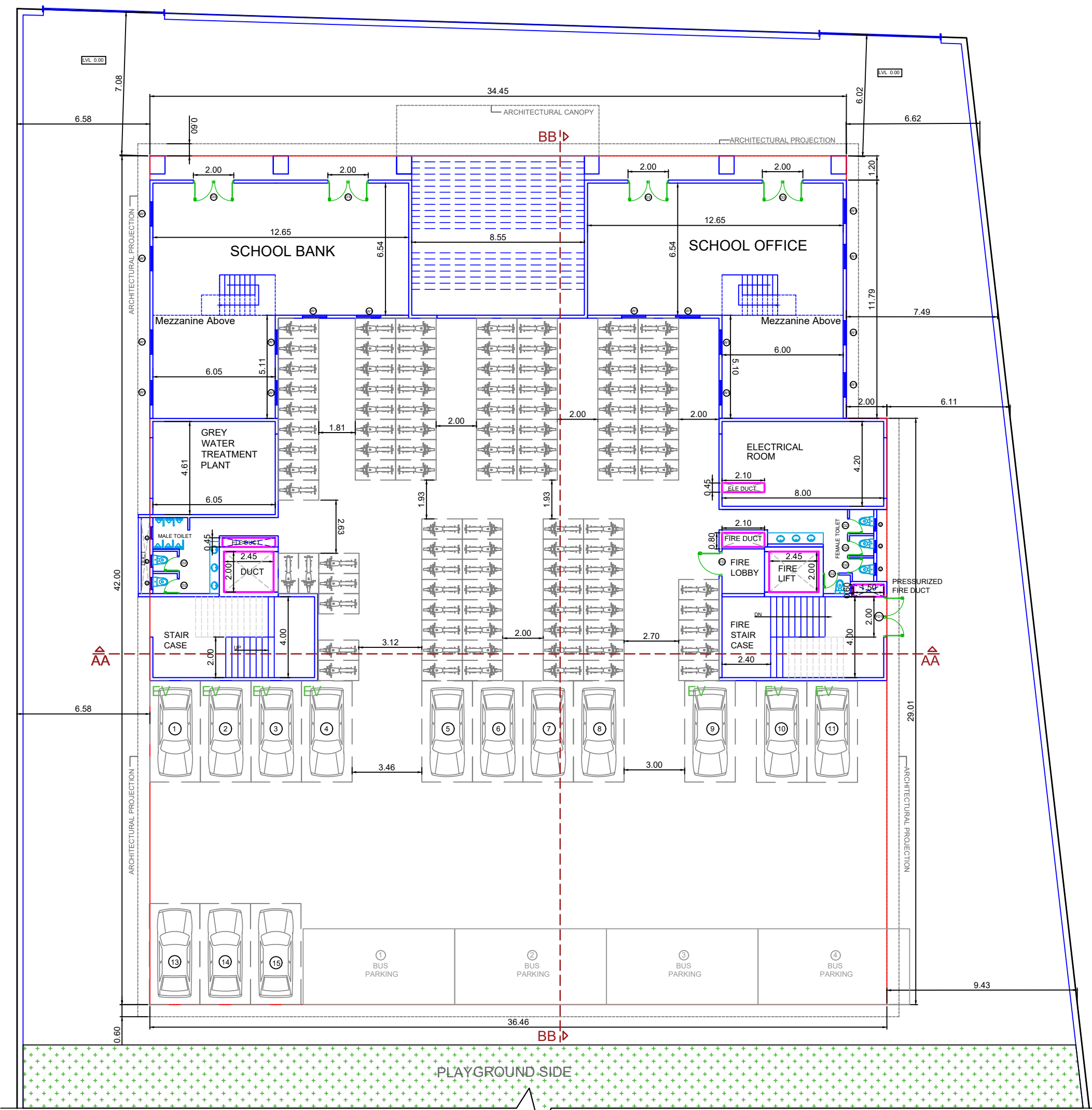
GROUND FLOOR PLAN WITH PARKING
